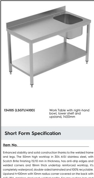
AISI 304 stainless steel spot welded profile. Square section legs and height adjustable feet (+20/+30 mm) in 304 AISI stainless steel. 400 x 500 x 250 mm welded and polished bowl supplied with an overflow pipe and 1,5" drain hole. 40 mm-thick lower welded shelf in AISI 304 stainless steel slots easily into place at a height of 200 mm from the floor. Lower shelf is compulsory to install the chest of drawers.
